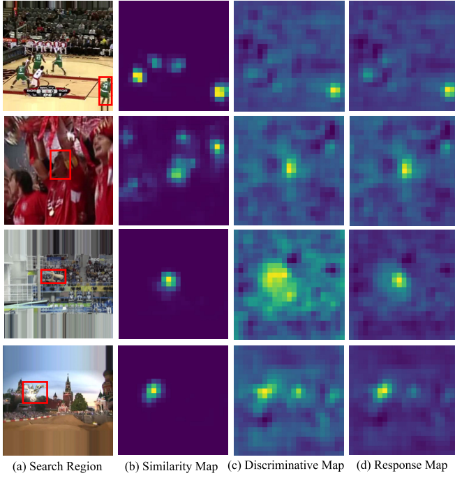
Fig. 3. Comparisons of similarity maps, discriminative maps and response maps produced from our framework on four examples. The final response maps can perform better target localization than both the intermediate similarity maps and discriminative maps.
