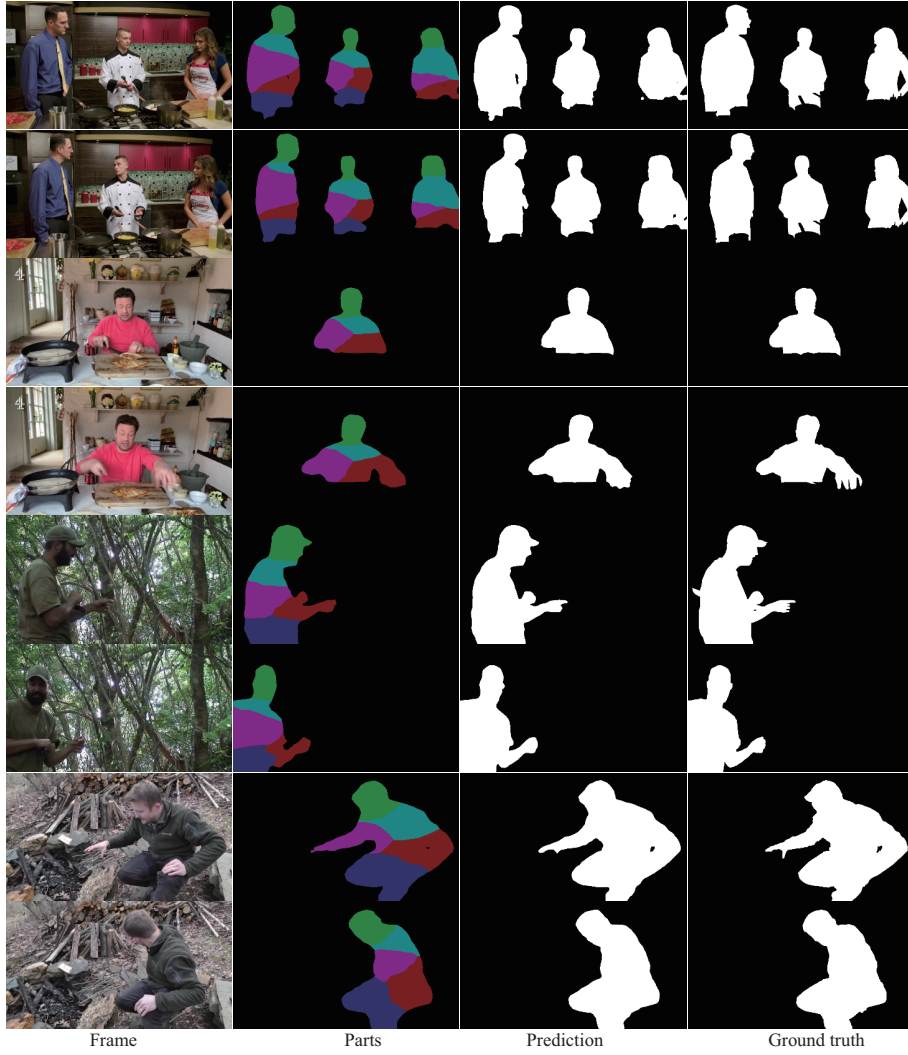
Figure 8 (Color online) Visual examples of decoupled parts and segmentation results of our PDNet on the test set of MVPS dataset.
